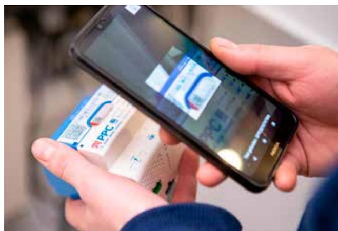
Fig. 3 - Registration process for a Smart Meter Gateway before installation: A PIN/TAN registration process for the installation of the Smart Meter Gateways implemented in Germany to improve the security of the smart grid information system (Photo: © PPC AG).
