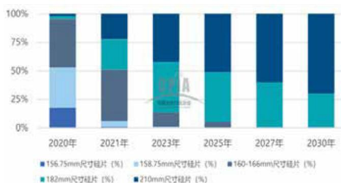
Fig. 6 - Trend of silicon wafers with different sizes.
